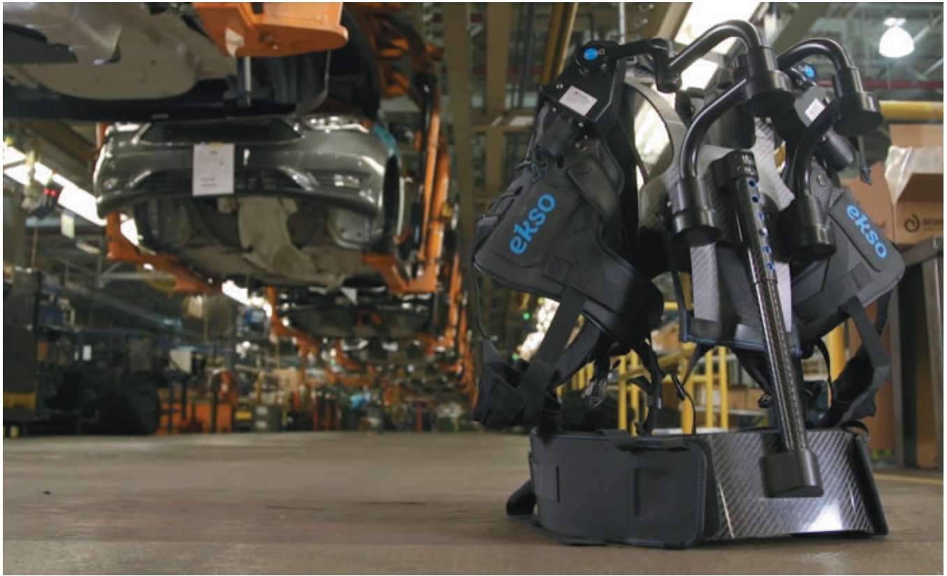
The EksoVest is worn by the construction worker and enables him to lift more overhead. PHOTO COURTESY OF EKSO BIONICS
