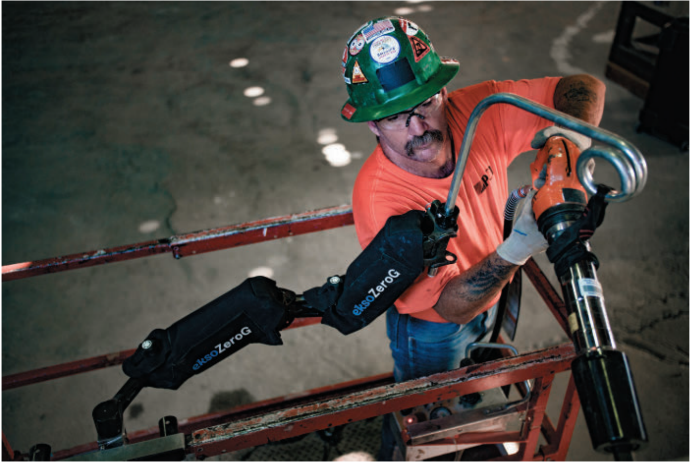
The EksoZero G helps in holding equipment overhead. PHOTO COURTESY OF EKS0 BIONICS
