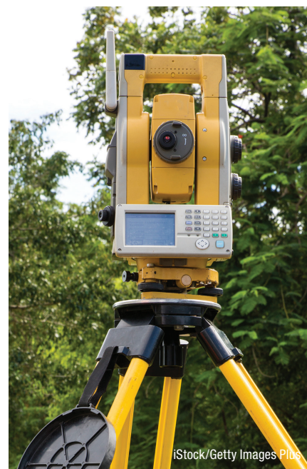
View of robotic total station.
