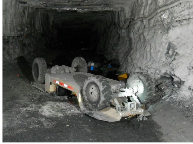
A miner was fatally injured while riding on a personnel carrier. The emergency stop was activated on an uphill grade, causing the personnel carrier to lose control, overturn, and pin the miner underneath.
