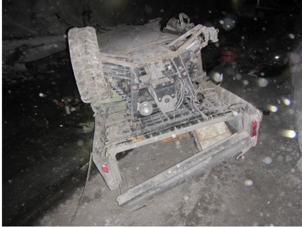
A miner was fatally injured while operating a personnel carrier. While traveling down a mine slope, the personnel carrier lost control, crashed at the bottom of the slope, and pinned the miner underneath.
