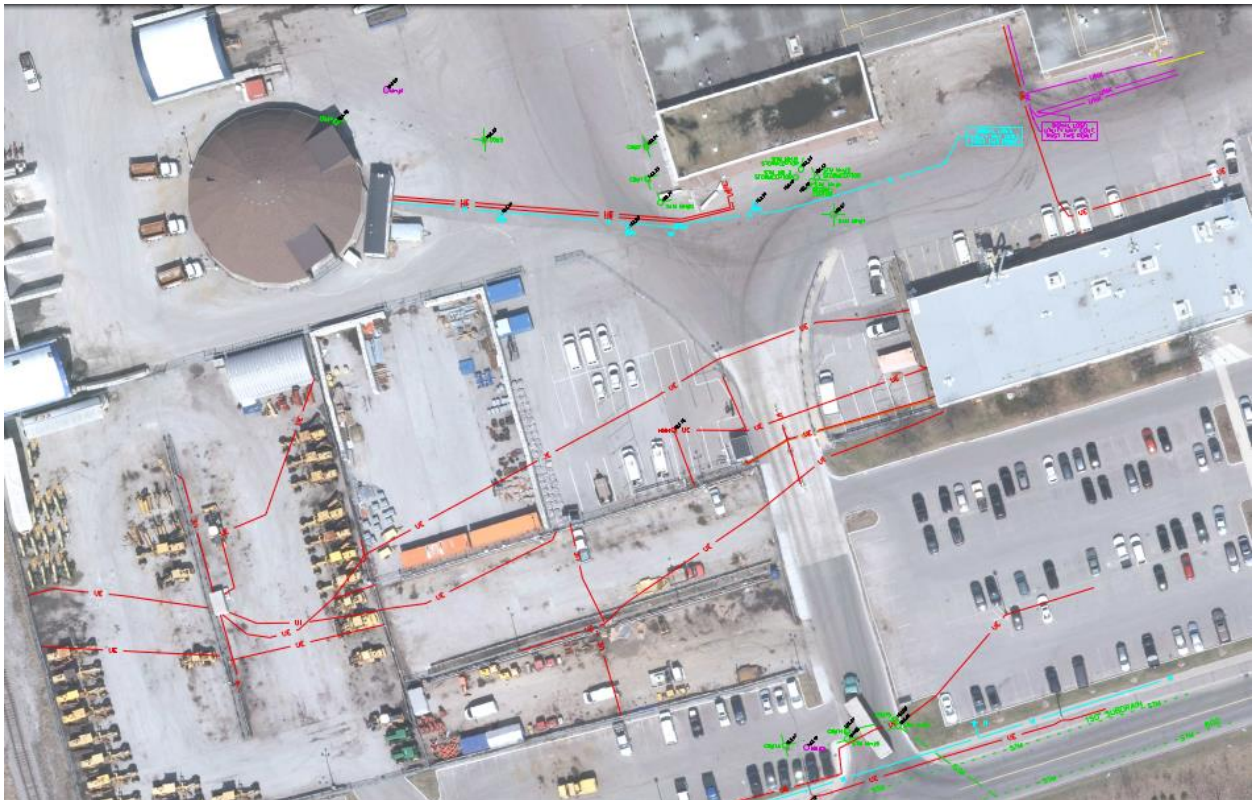
Fig. 1 – SUE project: Orthophoto base layer, with georeferenced Utility information shown.
