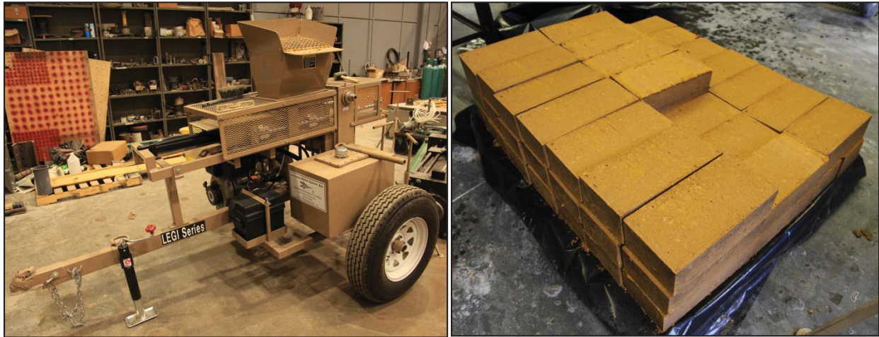
Figure 1. AECT Impact 2001A machine and example blocks
