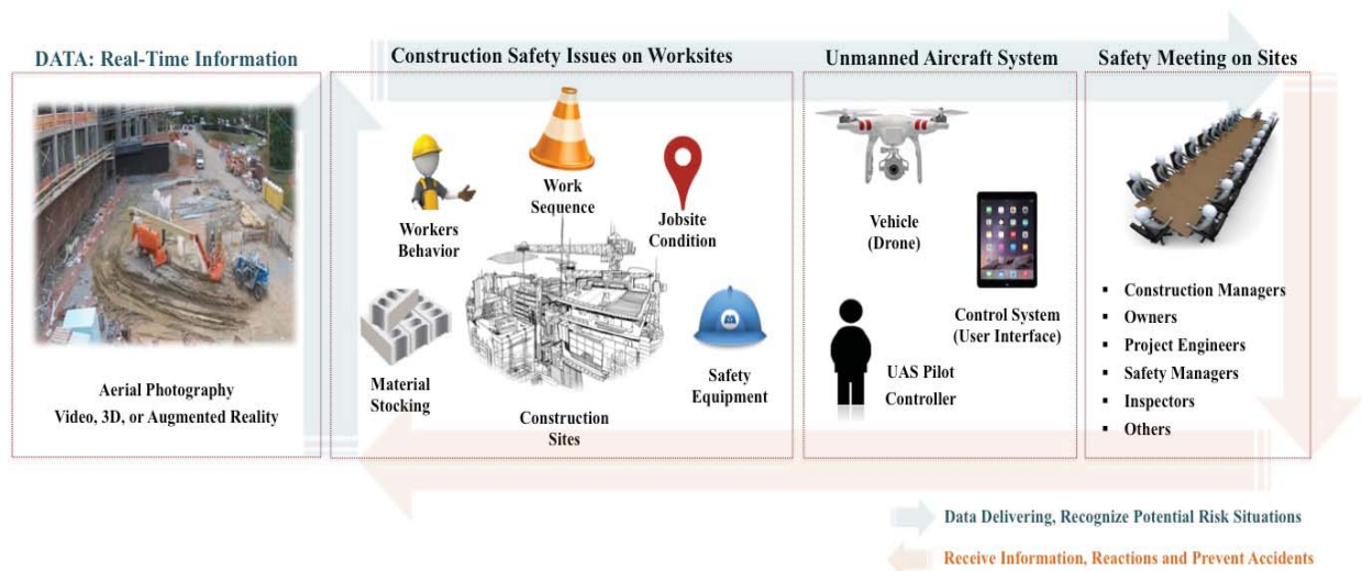
Figure 2. Concept of UAS-based safety monitoring
