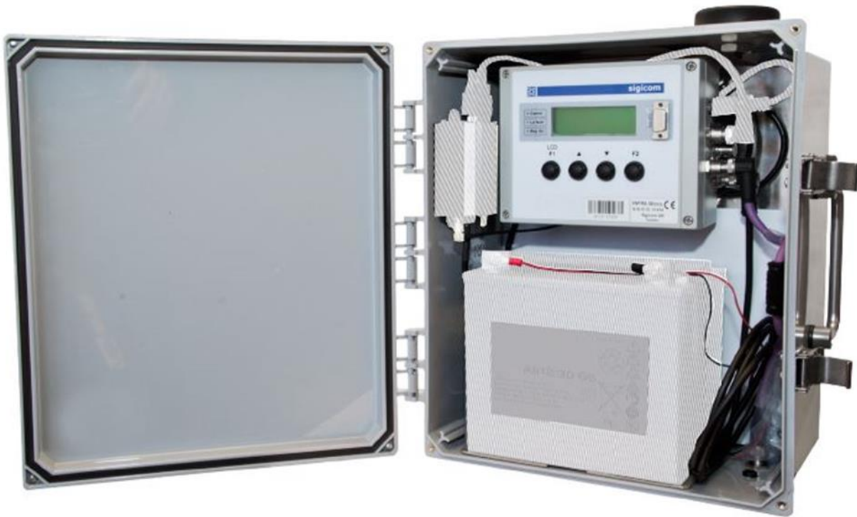
Example of One Long-Term Noise and Vibration Monitoring System used by Pinchin. Photo Courtesy of Sigicom August 9, 2017
