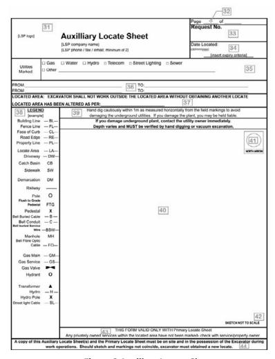
Figure 2 Auxiliary Locate Sheet
