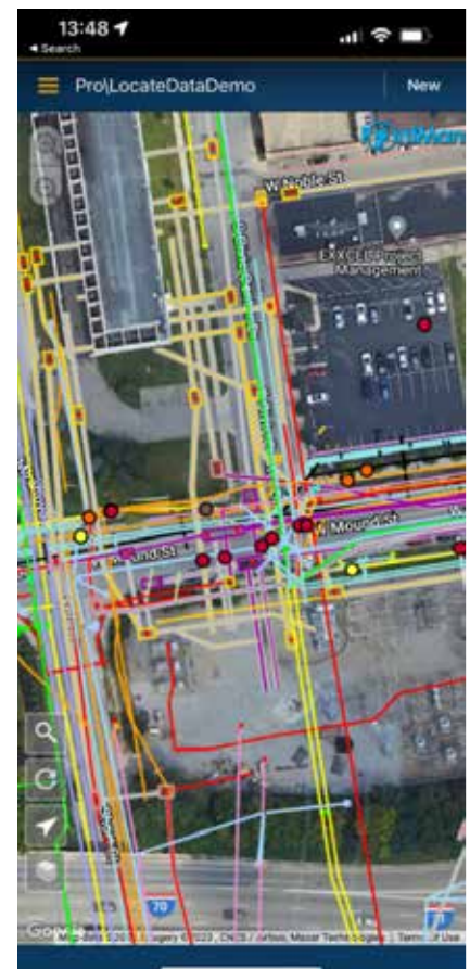
Figure 3. Screen shot of PointMan mobile field app depicting utility information at jobsite.
