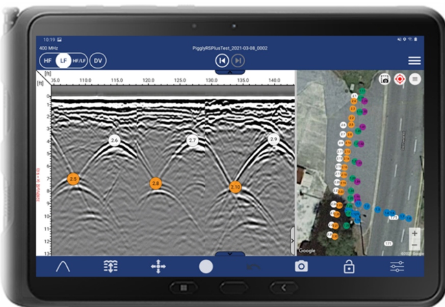
Figure 2. Screen shot of PinPointR GPR ViewPoint app. Utility targets marked with RTK GPS in real time.
