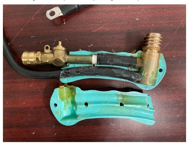
For example, when I was separating the casing, the silicon joined to the rubber shielding on the power line and tore it, exposing the bare wire within.
