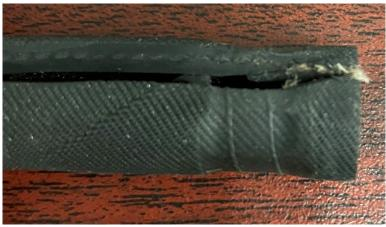
In addition to material concerns, there was a perforation in the outer protective layer for the hose caused by drilling out the hole for the screw which held the casing together. If this operation were to affect the hose itself, it could cause a rupture in the oxygen line.
