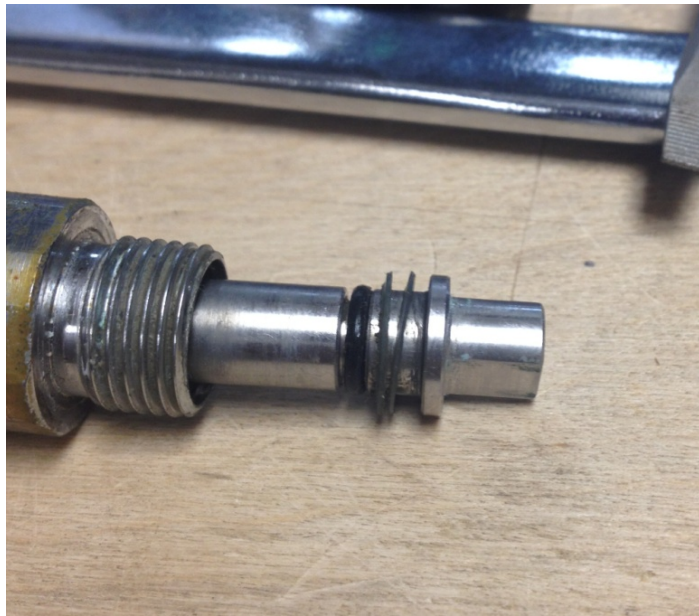
Extra washers on valve stem, valve not serviced
