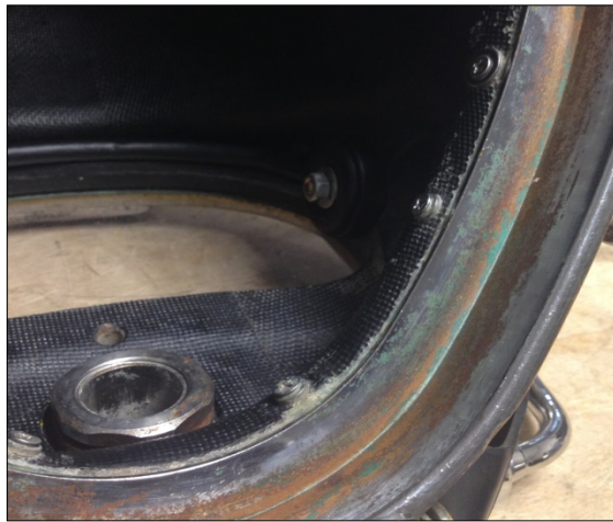
9 out of 10 head/chin cushion snaps broken or missing
