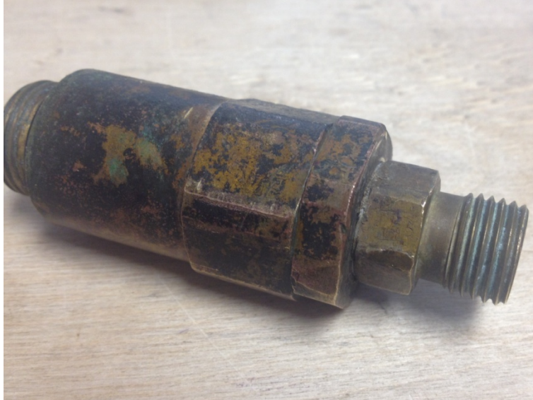
Umbilical adapter forced in too far; valve not serviced.
