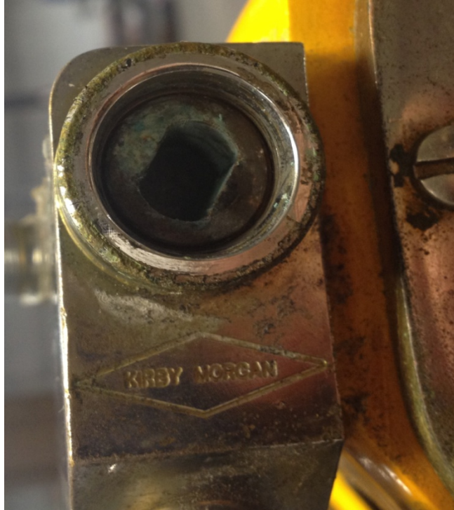
Mud and grit in the steady-flow valve, bonnet grinding in threads
