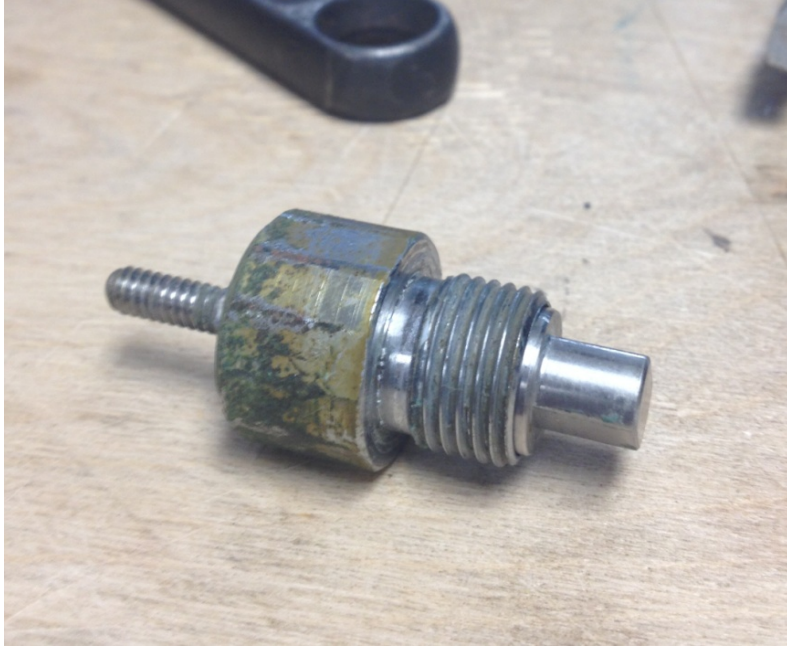
O-ring missing from steady-flow bonnet
