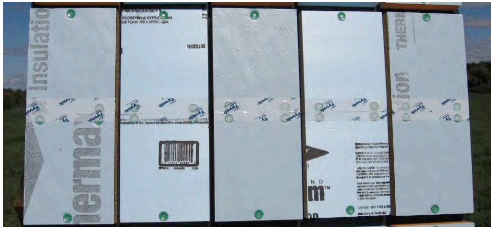
Figure 29 - Dupont Tyvek Tape Tests
