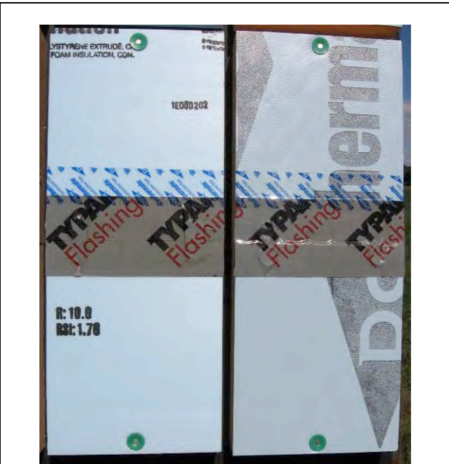
Figure 22 - Typar Tape with Termination Tape on ffPIC (right) and XPS (left)
