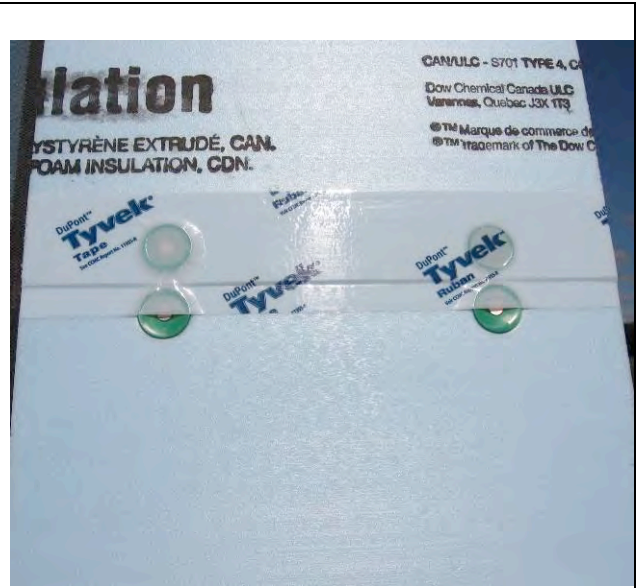
Figure 44 - Dupont Tyvek Tape on XPS - Large Sample
