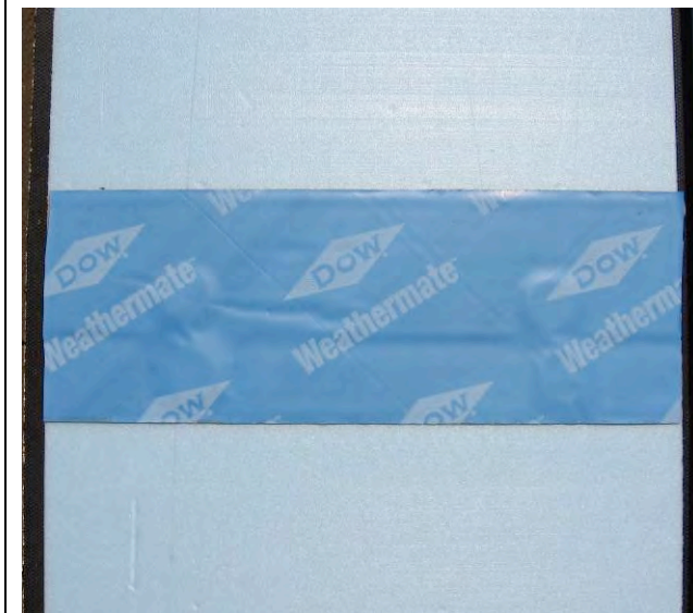
Figure 45 - Dow Weathermate Butyl on XPS - Large Sample
