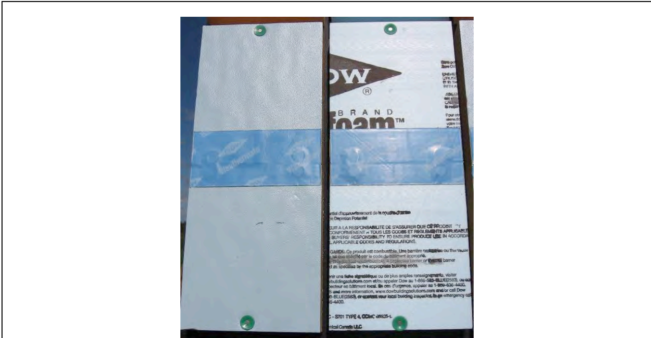
Figure 35 – Dow Weathermate Butyl on fPIC (left) and XPS (right)
