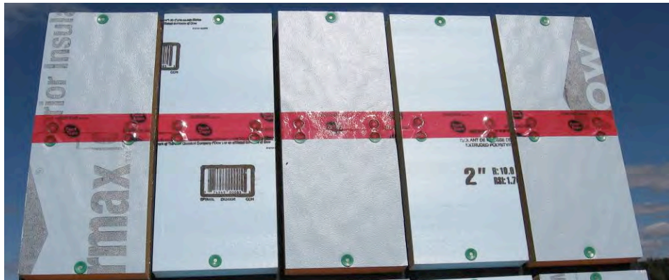
Figure 30 - Tuck Tape Tests
