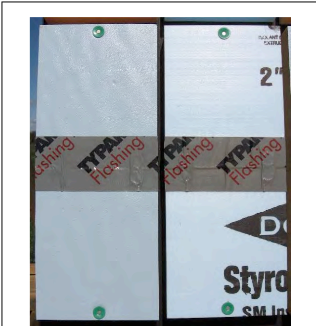
Figure 21 - Typar Tape on ffPIC (left) and XPS (right)
