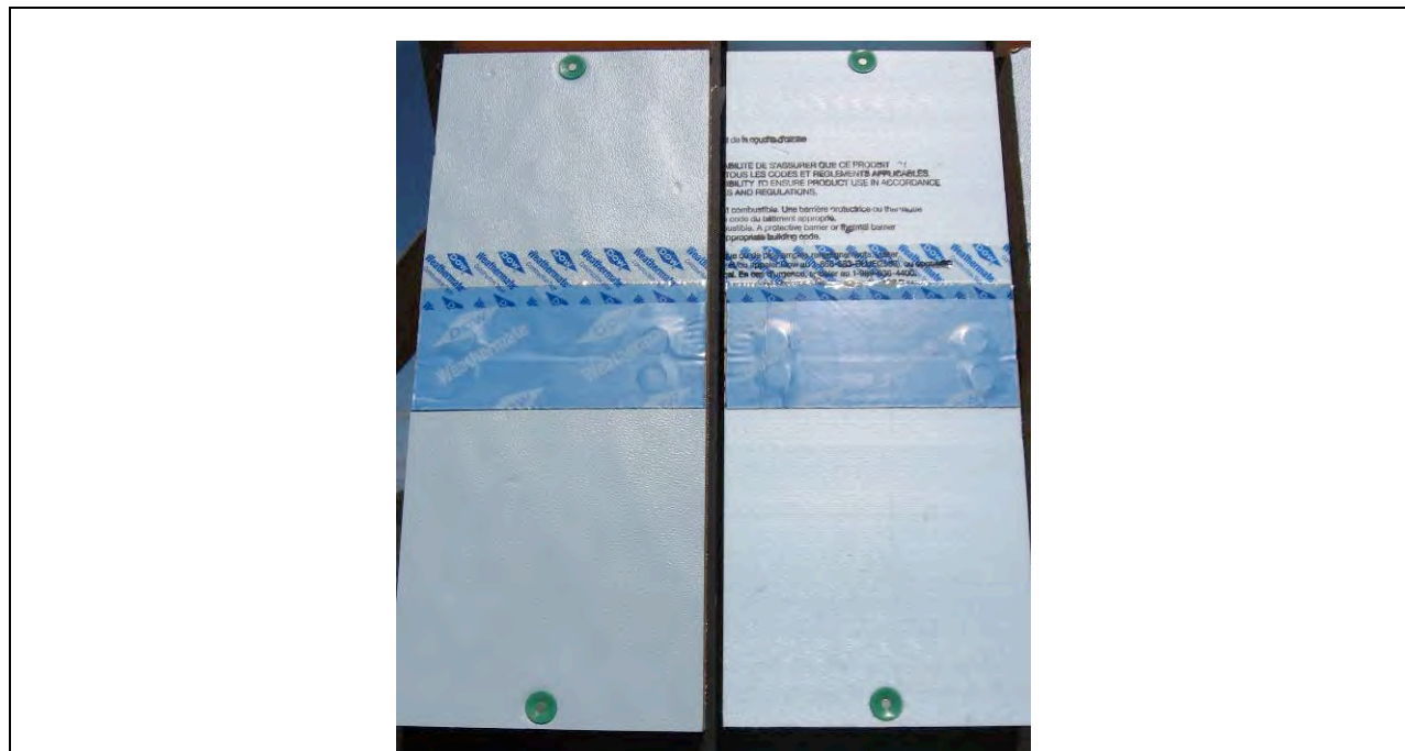
Figure 33 – Dow Weathermate Butyl with Termination Tape on ffPIC (left) and XPS (right)
