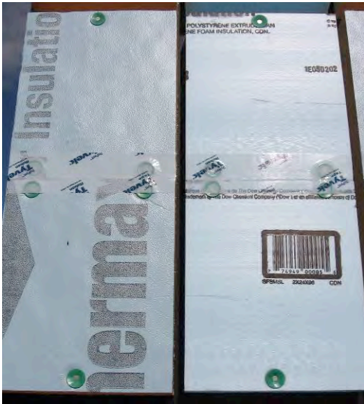
Figure 27 - Dupont Tyvek Tape on ffPIC (left) and XPS (right)
