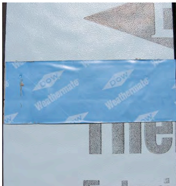
Figure 42 - Dow Weathermate Butyl on ffPIC - Large Test
