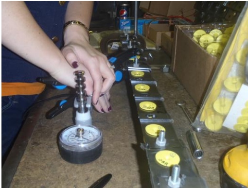
Figure 2. The insertion force required to apply the RFID tags was tested during the PAMI research team's test procedures.
