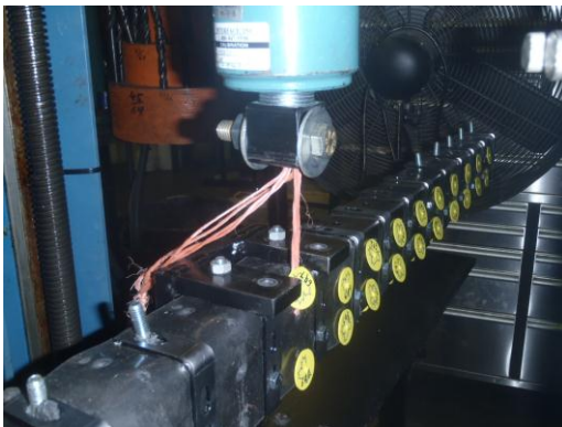
Figure 3. Shear force (above using twine), along with tensile and impact tests were conducted on six different brands of RFID tags during the PAMI test procedures.
