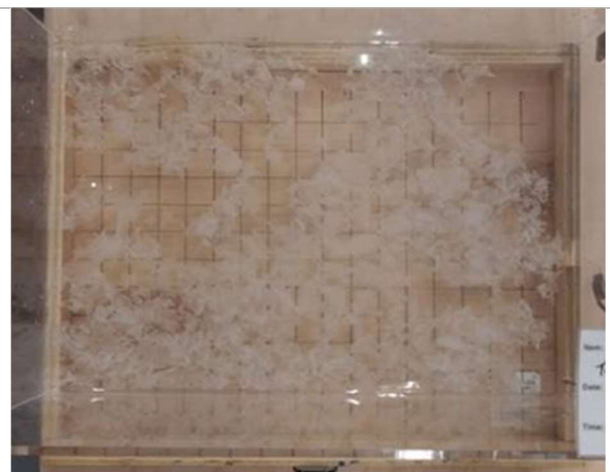
Figure 10- Example of Bathroom Tissue Disintegration After Testing
