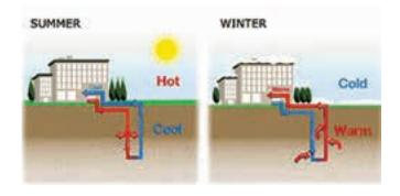
known as the ground loop heat exchanger. The heat exchanger located on the central campus is composed of 120, 500-foot-deep boreholes that are connected to form a single closed loop. The heat exchanger located at Eisenhower School is composed of 32,500-foot-deep boreholes.
