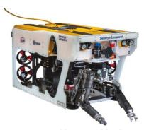
The 3000m rated Leopard is the most powerful electric underwater e-robotic system in the world, making it ideal for complex and demanding scientific tasks.
