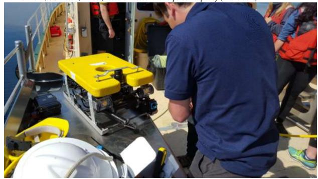
• Outland 1000 Remotely Operated Vehicle (ROV) with 244 meters (800 feet) of tether, single function manipulator, scanning sonar
