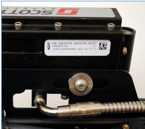
Location of Serial Number Label and manufacture date on Air-Pak 75 reducer
